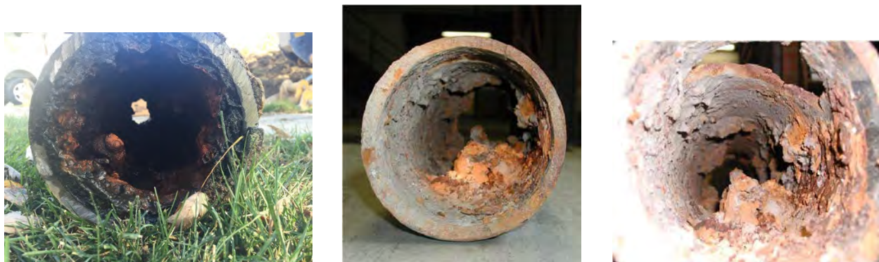
Picture 1 – 50+ Year-old 6 inch Cast Iron Water Mains
