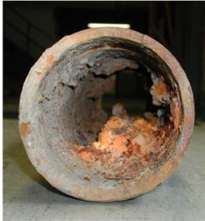
Picture 1 – 50+ Year-old 6 inch Cast Iron Water Mains
