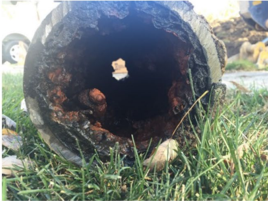
Picture 1 – 50+ Year-old 6 inch Cast Iron Water Mains
