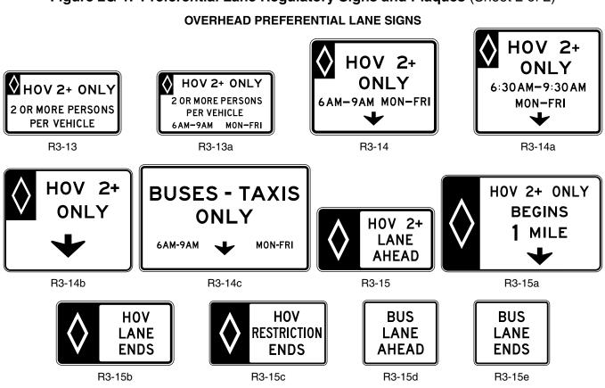
Figure 2G-1. Preferential Lane Regulatory Signs and Plaques (Sheet 2 of 2)
