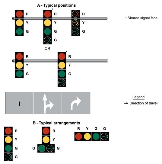
Note: Shared signal faces shall only be used for a protected-only mode right turn if the circular green and green right-turn arrow indications always begin and terminate together
