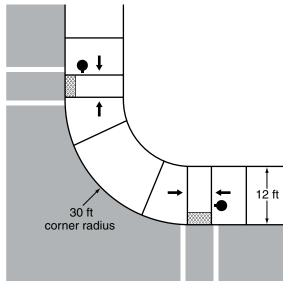
C - Parallel ramps with narrow sidewalk and tight corner radius
