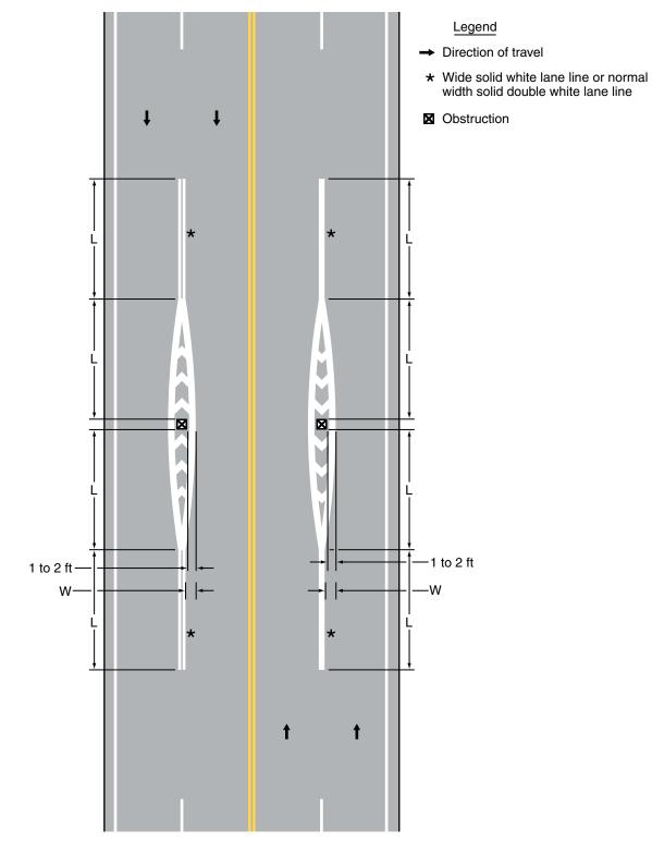
For speeds of 45 mph or more: L = WS For speeds of less than 45 mph: L =  $WS^2/60$ S = Posted, 85th-percentile, or statutory speed in mph W = Offset distance in feet
