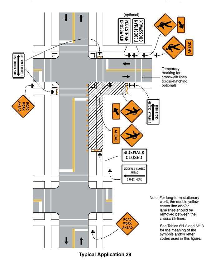
Figure 6H-29. Crosswalk Closures and Pedestrian Detours (TA-29)
