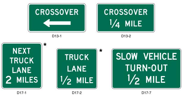
\* The words PASSING or CLIMBING may be substituted for the word TRUCK on the D17-1 and D17-2 signs.
