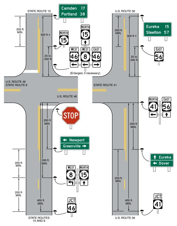
Note: The spacings shown on this figure are for rural intersections. See Sections 2D.29, 2D.30, 2D.32, 2D.34, 2D.40, and 2D.42 for low-speed and/or urban conditions.
