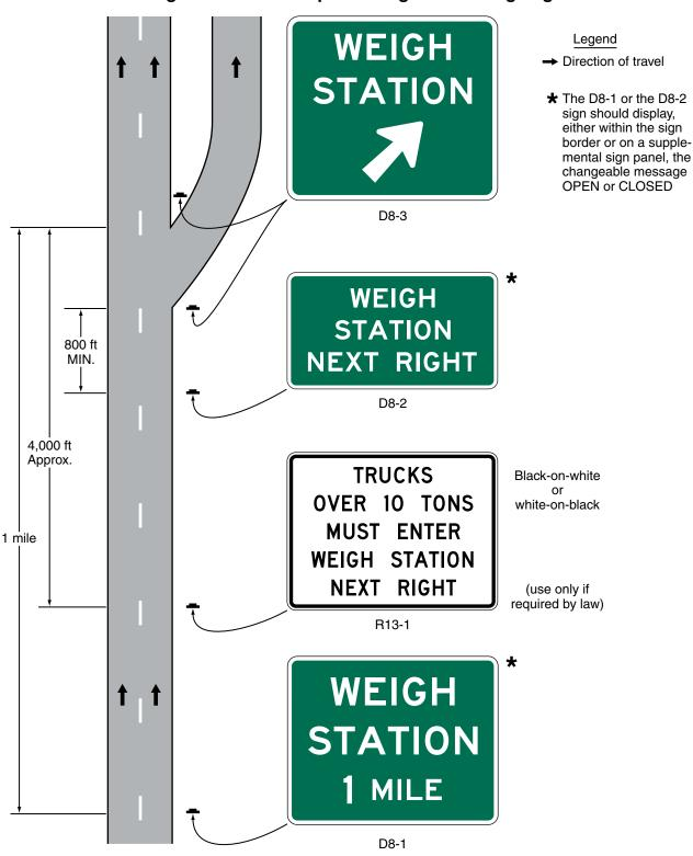
Figure 2D-17. Example of Weigh Station Signing
