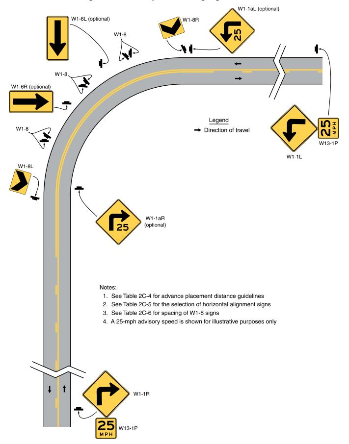
Figure 2C-2. Example of Warning Signs for a Turn
