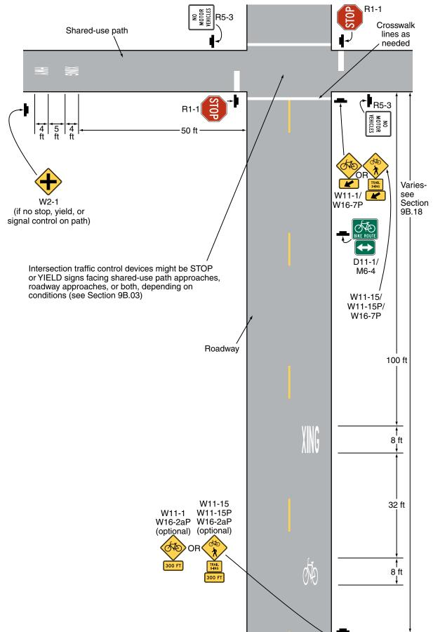
Route sign auxiliary plaques carrying word legends that are used on bicycle routes should have a minimum size of 12 x 6 inches. Route sign auxiliary plaques carrying arrow symbols that are used on bicycle routes should have a minimum size of 12 x 9 inches.
