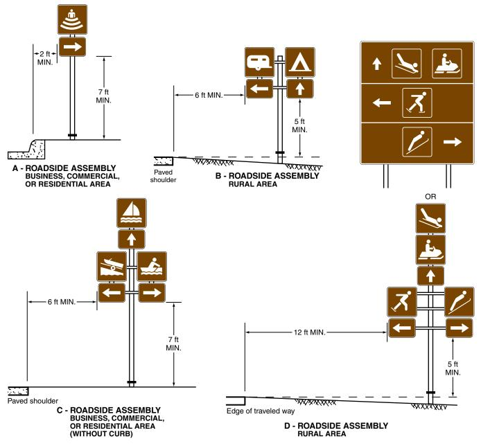
Note: See Section 2A.19 for reduced lateral offset distances that may be used in areas where lateral offsets are limited, and in urban areas where sidewalk width is limited or where existing poles are close to the curb.
