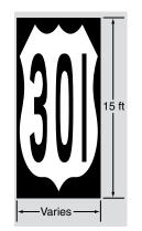
D - State Route Shield E - State Route Shield on dark pavement on light pavement
