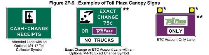
Optional flashing yellow beacons that are separated from any lane-use control signals for the lane (see Section 2F.16)
