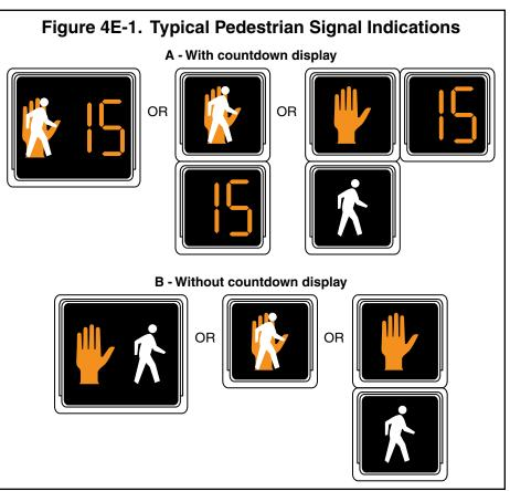
the symbols shall be either overlaid upon each other or arranged side-by-side with the UPRAISED HAND symbol to the left of the WALKING PERSON symbol, and a light source that can display each symbol independently shall be used.
