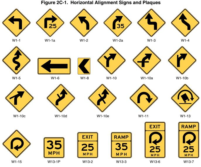
Note: Turn arrows and reverse turn arrows may be substituted for the curve arrows and reverse curve arrows on the W1-10 series signs where appropriate.
