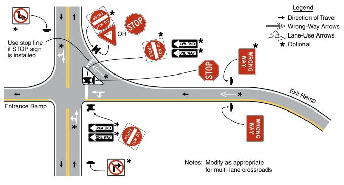
Figure 2B-19. Example of Application of Regulatory Signing and Pavement Markings at an Entrance Ramp Terminal Where the Design Does Not Clearly Indicate the Direction of Flow
