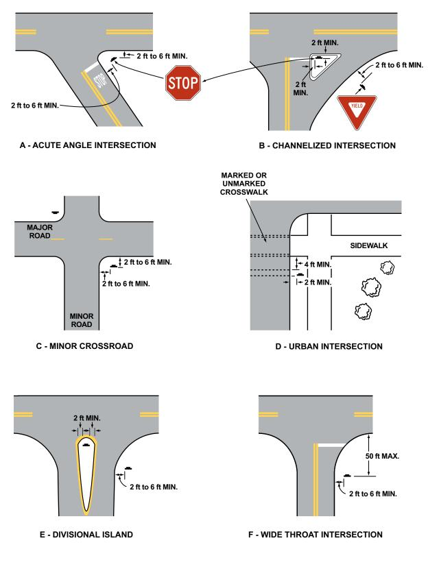
Note: Lateral offset is a minimum of 2 feet measured from the edge of the shoulder, or 6 feet measured from the edge of the traveled way. See Section 2A.19 for lower minimums that may be used in urban areas, or where lateral offset space is limited.
