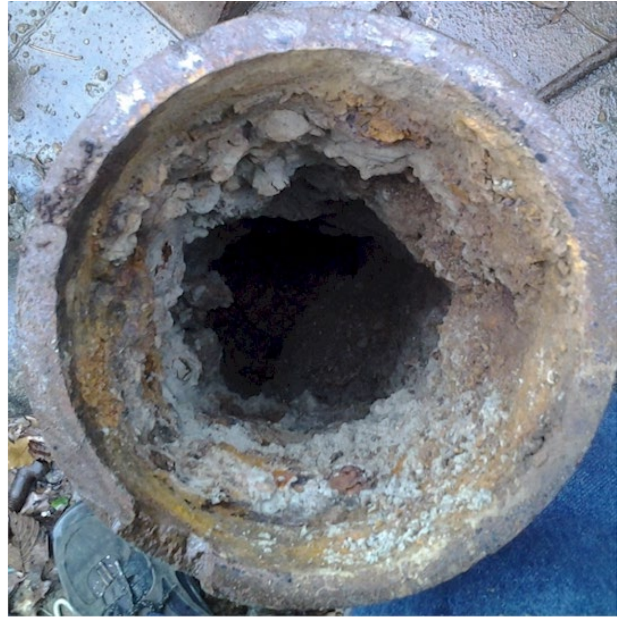
Cast iron water mains with interior corrosion – ours will look like these
