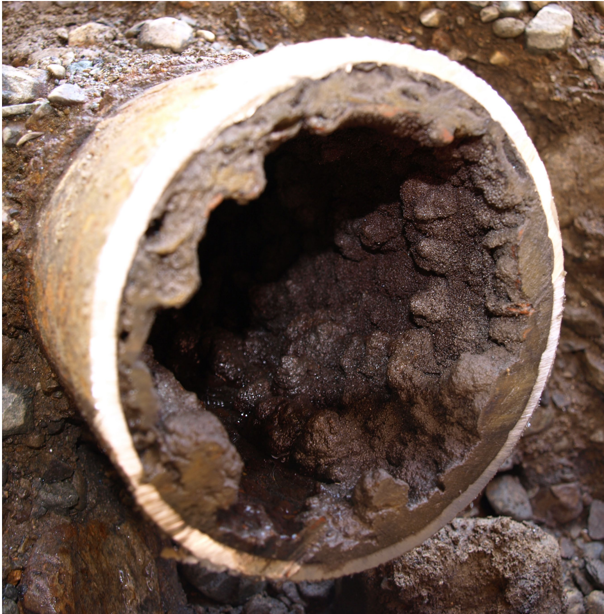
Cast iron water mains with interior corrosion – ours will look like these
