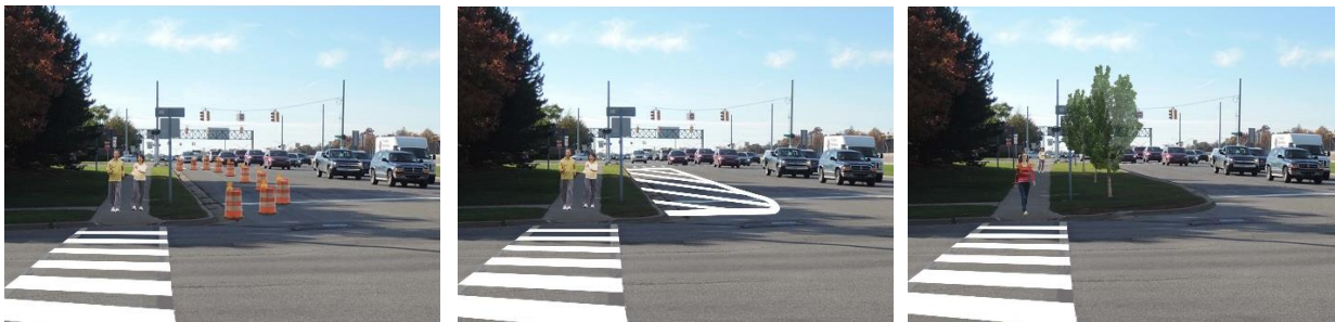
Figure 1: This three step diagram demonstrates short-term techniques for testing the removal of excess roadway before the eventual capital investment of moving a curbed parkway.
